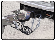
Chains and cables ensure safe towing
