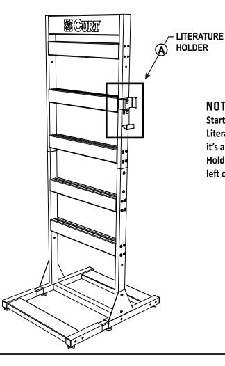
NOTE: if only one CrossBar is installed on Starter Kit, and/or if you need to offset Literature Holder to one side of Starter Kit, it's also acceptable to secure Literature Holder using only 2 bolts through either the left or right column of key-holes.
