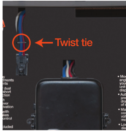
12. Secure the quick plug down with the twist tie provided
