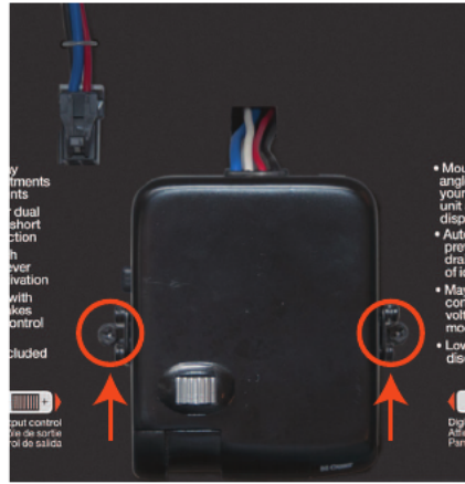
14. You can now attach the TriFlex to the mounting bracket
