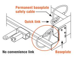
Note: Base plate safety cables are not a replacement for safety chains connecting the tow vehicle to the towed vehicle.
