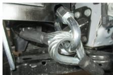
Use the included cable tie (#8) to reattach the temperature sensor to the plastic loop below the radiator on the driver-side of the vehicle.
