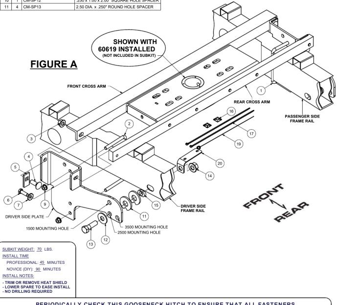
PERIODICALLY CHECK THIS GOOSENECK HITCH TO ENSURE THAT ALL FASTENERS ARE TIGHT AND THAT ALL STRUCTURAL COMPONENTS ARE SOUND.
