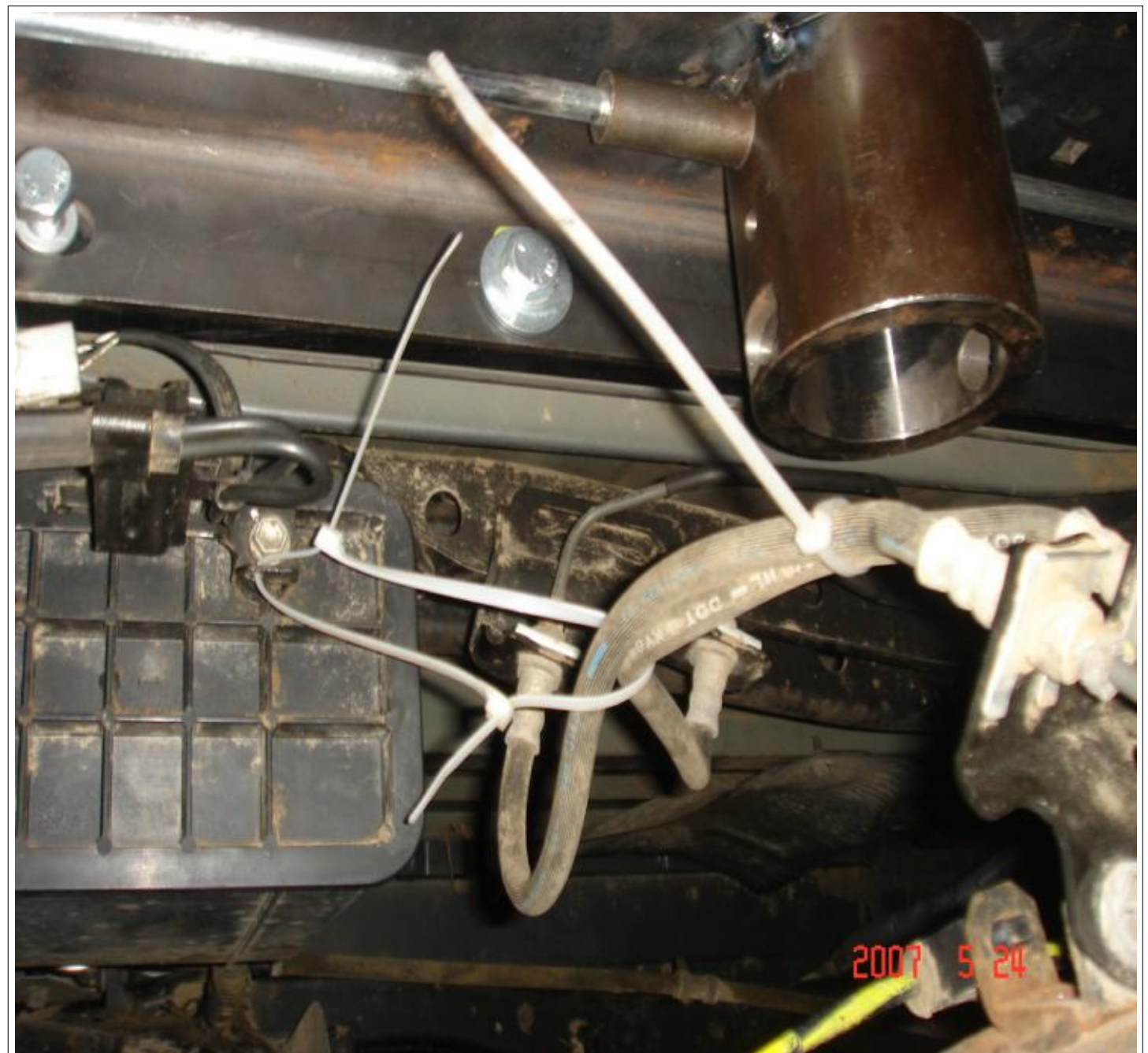
MODIFIED BRAKE LINES USING CABLE TIES
