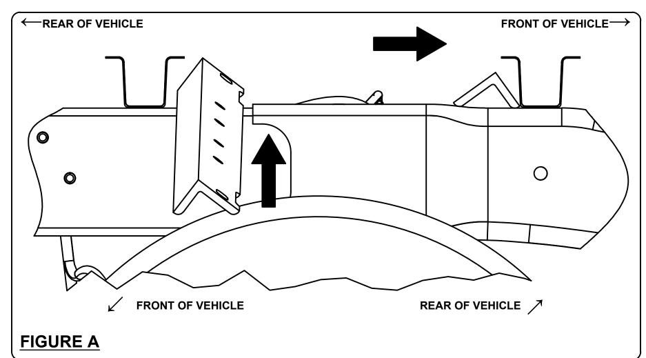
into position. The cross arm can be used as a lever to add additional bend to the flange, if needed. Insert the cross arm in the location shown in FIGURE A until it spans the frame rails. Slide the cross arm forward so that it is next to the forward bed support.
