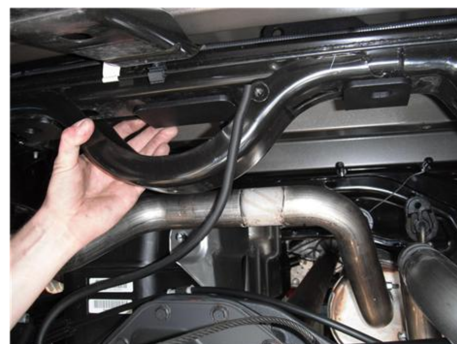
Figure 8.1: Axle Vent Hose Relocation
