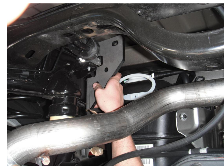
Figure 6.5: Driver side plate as viewed from floor up toward driver side frame. (Fuel tank is not shown.)
