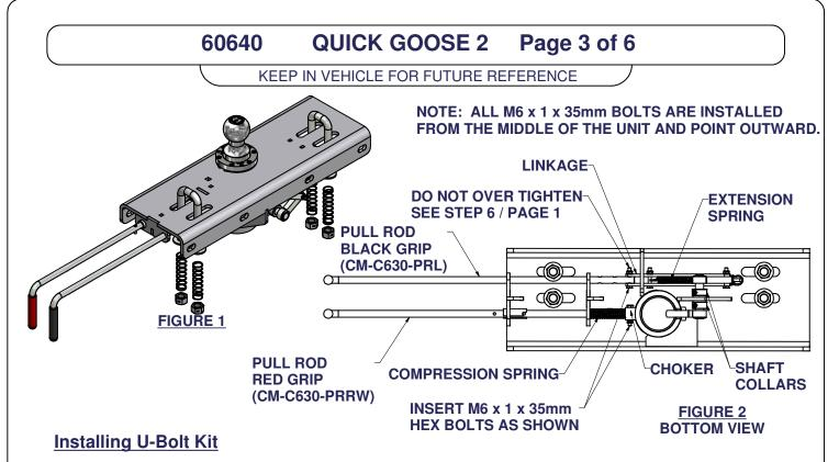
1) After the 60640 is centered and torqued to specifications, from under the bed, using the 60640 as a template, mark (4) holes within the (4) slots to be drilled for the Safety Chain U-Bolt Kit attachment.
