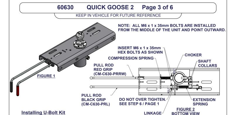
1) After the 60630 is centered and torqued to specifications, from under the bed, using the 60630 as a template, mark (4) holes within the (4) slots to be drilled for the Safety Chain U-Bolt Kit attachment.
