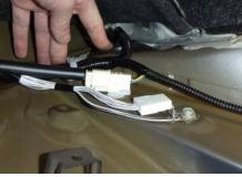
Reinstall the taillights and tighten the zip ties on the green wire. Secure any excess wire so that it is not drooping or dangling, but not so tight that it causes unnecessary strain to the wire which could lead to breakage over time.
