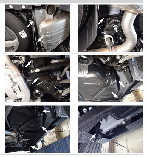
Pull the 4-flat up between the inner and outer fender route under the weather strip around the back of the engine compartment to the front of the vehicle.
