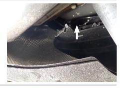
Route the housing with the yellow wire above the bumper mount and along the bumper to the driver side. Zip tie as needed along the bumper. Route above the driver-side bumper mount.
