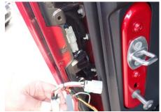
Route the green wire over the vehicle frame on both sides of the vehicle over to the passenger side. Zip tie as needed to the rear bumper.
