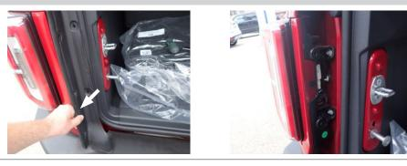
Locate the taillight housing and separate the connectors, taking care not to damage the locking tabs. Repeat this on the other side of the vehicle.
