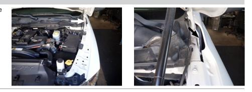
Route the 4-flat along the driver-side inner fender. Mount the 4-flat in the front of the vehicle under the hood.
