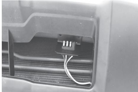
12. With the 4-flat extension plugged into the RV harness on one end and the motorhome on the other, test that the functions work on the Honda Element. These functions will only work on the brake/tail combination lamp.
