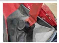
Remove the one bolt under each taillight opening securing it to the bumper cover.
