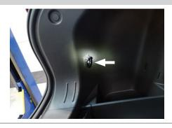
Use a trim tool loosen the sidewall on the driver side. Locate the taillight housing in between the body and the wall panel. They will be secured to the side wall with push fasteners.
