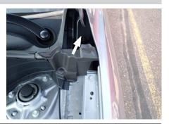
Route under the foam trim and under the front fender ledge to the front of the vehicle along the rear of the headlight. Mount the 4-flat in the engine compartment towards the front of the vehicle.
