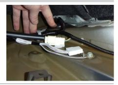
Test the harness with a separate vehicle by plugging the RV harness 4-flat to a second vehicle with a working mating 4-flat. Test that the stop, turn, and taillight functions work properly before completing the install.
