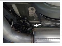
After routing past the muffler, keep the harness up close to the body of the vehicle away from the rear suspensions. Route along the fuel tank. Once at the brake lines, stay between them and the center of the vehicle until routing up into the engine compartment.
