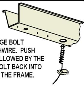
ATTACH FISHWIRE TO CARRIAGE BOLT AND SLIDE SPACER ONTO FISHWIRE. PUSH THE BOLT THRU THE HOLE FOLLOWED BY THE SPACER (AS SHOWN). PULL BOLT BACK INTO POSITION, PROTRUDING FROM THE FRAME.
