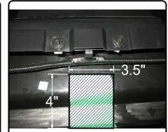
4. Raise side plates into position and loosely secure (4) hex flange nuts onto existing bolt plates or 1/2-13 x 1 3/4" bolts. Fishwire supplied (2) 1/2-13 x 1 3/4" carriage bolts and CM-SP10 spacers through front of driver and passenger side frame rails and out slot on bottom of frame rail. Loosely secure 1/2-13 hex flange nuts onto carriage bolts.
