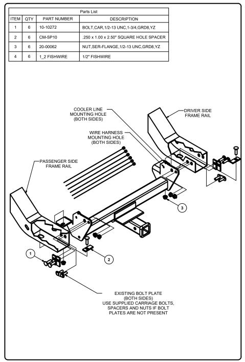
. Use 18mm socket and ratchet to remove driver and passenger side fascia brackets and return to owner. If present the existing bolt plates will fall out in front of frame rails. Temporarily move electrical harness off of frame rail. **NOTE:** If oil cooler lines are present remove by unclipping attachment from frame rail.
