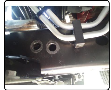
2. Fishwire (2) bolt plates removed in STEP 1 through original holes on inside of frame rails.
