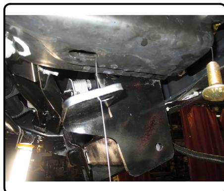
5. Secure all hardware and torque all 1/2" hardware to 110 ft-lbs and all M12-1.75 to 86 ft-lbs. Reconnect electrical harness through hole in driver side plate.
