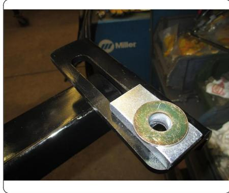
4. Insert one (1) M12 hex bolt with one (1) 1/2" conical toothed washer through side plate, CM-SP52 spacer and 1/2" flat washer into each rear most weldnut.
