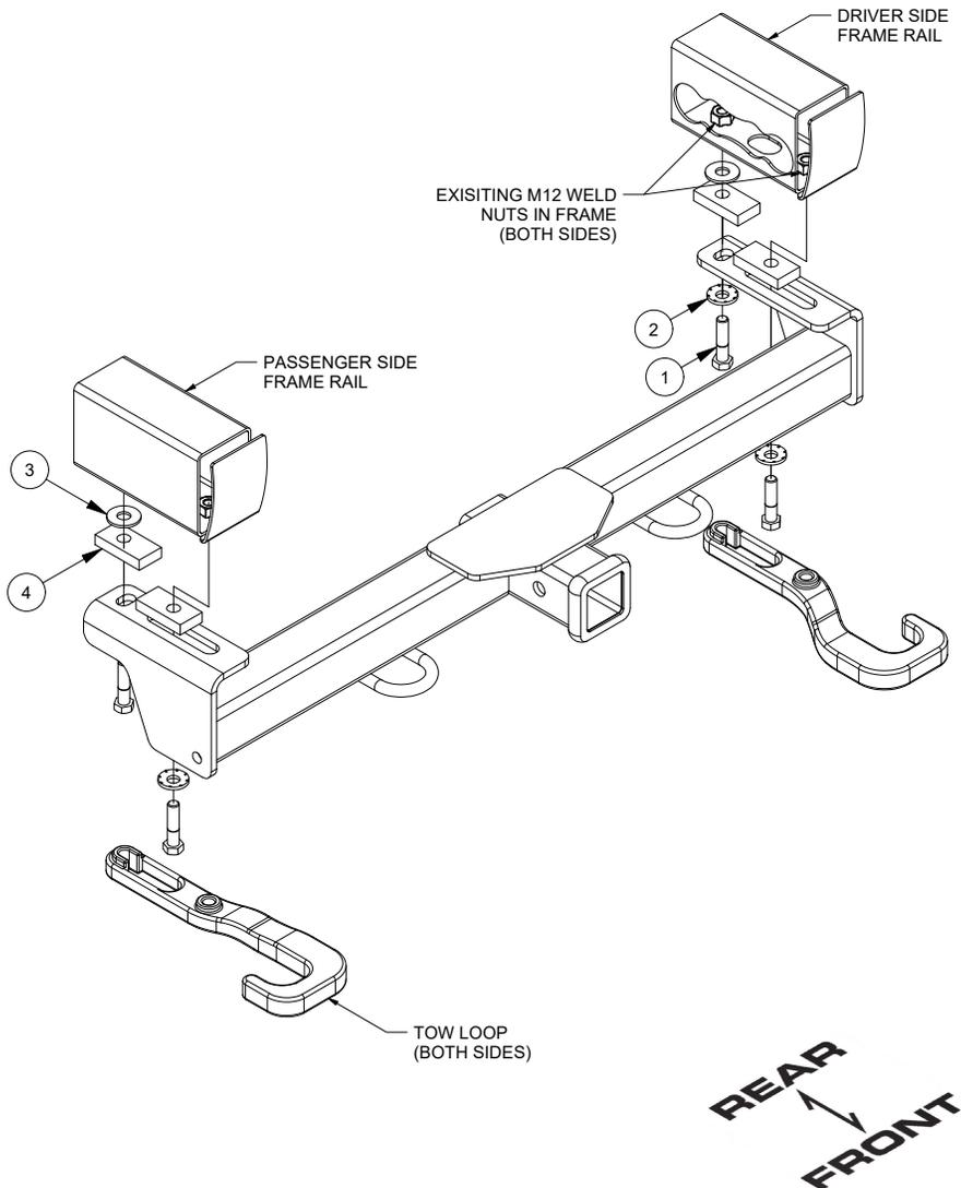
1. Remove two (2) hex bolts and one (1) tow loop from bottom of each frame rail and return to vehicle owner. These will be replaced with the included M12 hardware.
