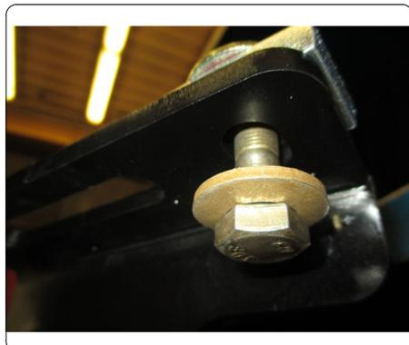
5. Secure all M12 fasteners with socket wrench. A 19mm end wrench may be used to secure forward most bolt.
