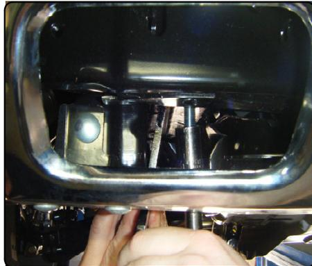
6. Assemble center hitch to side plates using 7/16" hardware as shown in ILLUSTRATION and pictures below.
