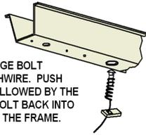
5. After fishwiring hardware into frame raise side plates and tow hooks into position and bolt to frame using spacers, 1/2"-13, and M12 hardware. (Finger tighten only).
