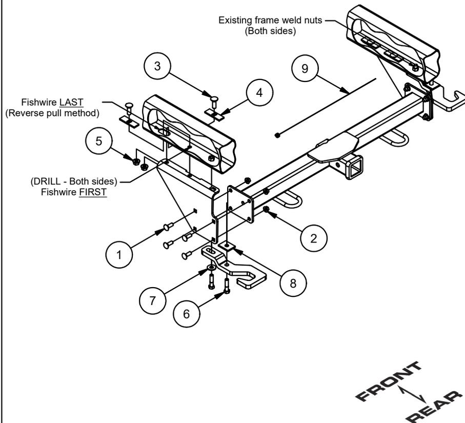
1. Remove tow hooks and set aside for later reattachment. Hardware to be returned to vehicle owner and will not be reused.
