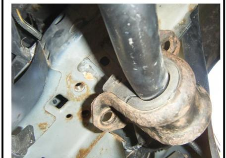
2. Slide drivers side plate into place, inbetween frame and bushing retaining bracket. Reinstall the 12mm bolts. Leave hardware loose until all bolts are installed.
