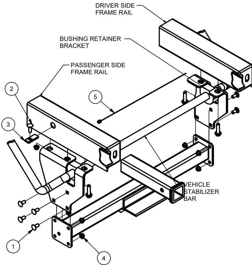
1. Remove front stabilizer bar bushing retaining bolts (save bolts for reinstallation)
