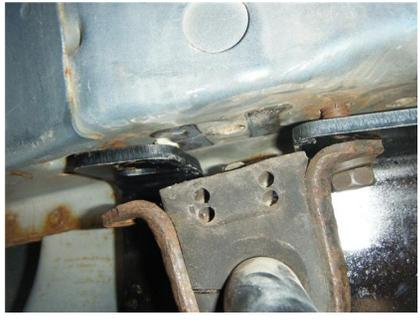
4. Locate back slot in passenger side plate and drill 1/2" dia. hole into frame. Fishwire CM-SP2 spacer and 7/16 x 1.25" long carriage bolt through hole on outside of frame.
