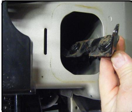
9. Fishwire (2) carriage bolts and spacers through the front of each frame rail, as shown below and in the illustration on sheet 2.
