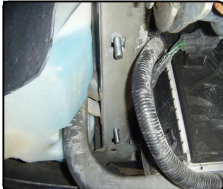
13. Using the fishwires on the carriage bolts as a guide raise hitch into position. (Rubber guards will need to be temporarily flipped out of the way on 2010 models)
