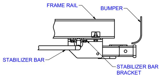
INSTALLED HITCH POSITION
