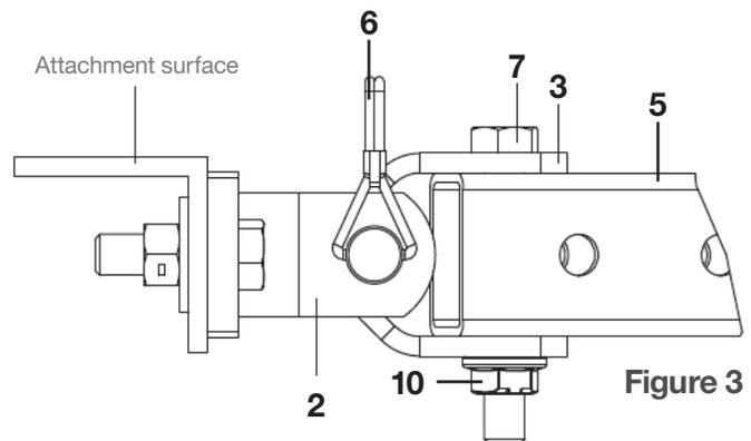
Tighten hardware until contact is made with both sides of the tow bar arm. Tow bar arms must swing freely; back off slightly if necessary.
