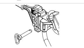
To check if arms are properly loaded, lift up on the snap-up bracket until resistance is felt. The handle should be appoximately be at 30°. If you are experiencing load restistance prior to 30°, adjust the tilt of the horn until you reach the correct angle. This will help with proper pin installation on uneven terrain
