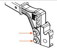
Run the set screws inside the horn to make the horn parallel to the shank (no tilt).
