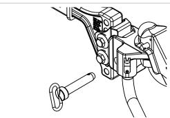
Snap-up one snap-up bracket at a time, ensuring that the clevis pin is installed before taking pressure off of the handle. Measure the front and rear bumper again. If you're within 1/2" of the measurement found at the top of step 5, no further adjustment is needed.
