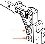
Run the set screws inside the horn to make the horn parallel to the shank (no tilt).
