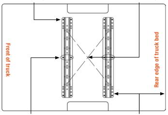
Each base rail must have a bolt in either of the marked holes. Check for obstructions before drilling Rear edge of truck bed to rear edge of base rail
