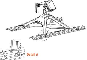
If installing new base rails, follow the instructions provided by the rail manufacturer for proper placement, alignment and spacing per your vehicle's year, make and model. If the 5th wheel is being mounted to existing base rails, and alignment issues arise, it may be necessary to proceed as follows:
