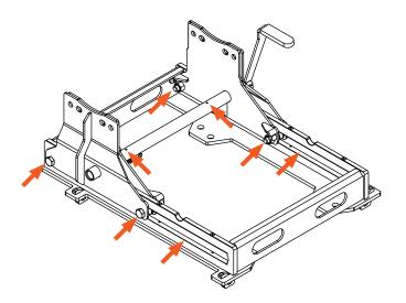
Prior to towing, ensure all components and hardware are structurally sound and secure. Periodically check the torque to ensure no fasteners have become loose.
