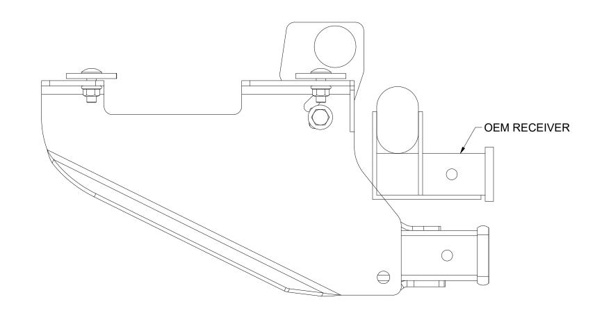
**INSTALLED HITCH POSITION**
