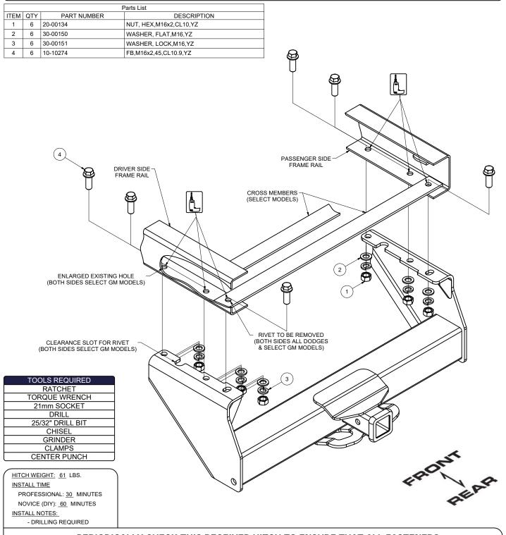
PERIODICALLY CHECK THIS RECEIVER HITCH TO ENSURE THAT ALL FASTENERS ARE TIGHT AND THAT ALL STRUCTURAL COMPONENTS ARE SOUND.
