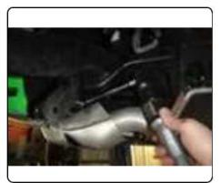
3. Remove the (2) existing hex bolts from the frame on both sides of the
