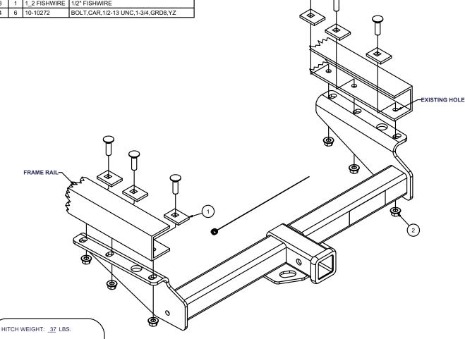
INSTALL TIME: <u>30</u> MINUTES INSTALL NOTES: ENLARGE EXISTING HOLES TO 1/2"
