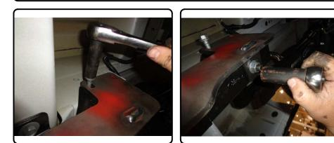
4. Torque M12 fasteners to 90 ft-lbs and all 1/2" fasteners to 110 ft-lbs. Re-install spare tire if lowered.
