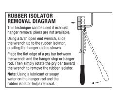
Lower the exhaust by unhooking the three (3) rubber isolators, two (2) by the muffler and one (1) towards the front of the vehicle.
