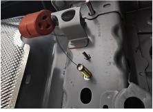
Use tin snips to make two (2) cuts in the center of the heat shield as shown. Bend the area between the cuts further so it is bent back onto itself.
