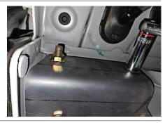
Reinstall the exhaust heat shield, slightly bending as needed to provide clearance for the hitch reciever.
