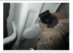
Using a die grinder with a carbide burr, enlarge the round hole in the bottom of the frame rails between the weld nut and plug clip slot to allow for the 7/16" carriage bolt and square hole spacer to pass through.
