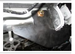
Raise the bumper fascia support back into position with the supplied tube spacers (#5) aligned with the small weldnuts, between the support and the frame rail.
