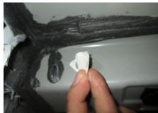
Thread the fishwire through the supplied 9/16" washers (#7) and into the forward holes in the hitch. Gently raise the hitch into position with the main body tube resting on the bumper fascia area.
