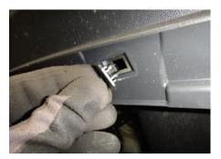
Use a T-25 torx bit to remove the screws from the rear fascia panel, one on each side of the rear lift gate below each taillight. Use a panel trim removal tool to remove the black plastic taillight cover located next to the taillight. Remove the two screws from the rear driver-side wheel well using a T-25 torx bit.
