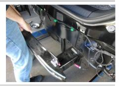
Raise the hitch and bumper beam into position and secure with the supplied M8 hex bolts (#1) and 3/8" conical-toothed washers (#2). Torque hardware to 23 ft-lbs.
