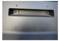
Carefully separate the wheel well trim, starting from the rearward-most part of the wheel well, working upward.
