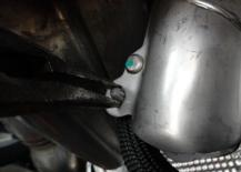
Lower the exhaust by removing two bolts from the exhaust support using a 16mm socket. Remove two torx-head bolts securing the exhaust in place. There will be one torx-head bolt on each side of vehicle.
