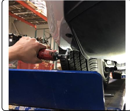
4. Gently remove rear fascia starting from the outside and releasing press-in tabs along the top portion of fascia. Unclip electrical harness and set aside rear fascia for reinstallation.
