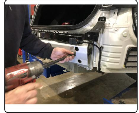
b. On 2021 and newer models there are (5) nuts, ((3) on driver side and (2) on passenger side) each side attaching the bumper beam and (6) nuts, (3) on each side attaching the bumper beam plates. Return bumper beam plates to vehicle owner.
