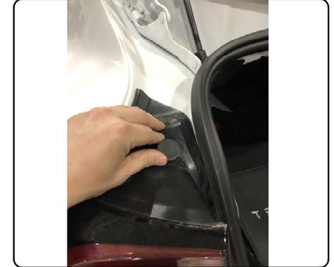
2. To remove taillight locate and remove (2) nuts, on each side, using 8mm socket. Unplug electrical harness and gently remove taillight. Set aside taillight for reinstallation. Remove exposed fascia screw using 10mm socket, on each side.
