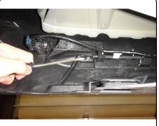
2. Remove (4) bolts and (2) nuts holding the bumper beam in place. Save the nuts for reinstallation in Step 3. Note: Bumper beam will be held up by vehicle studs on each side.
