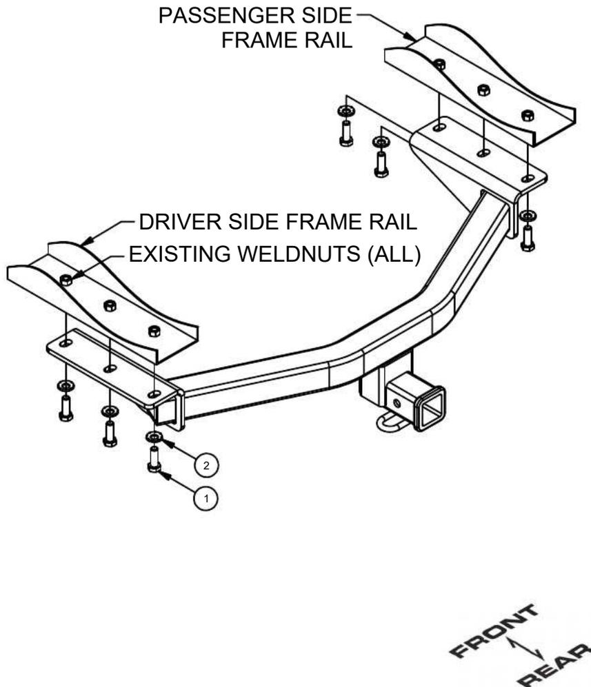
1. Raise hitch into position and secure with the provided M14 bolts and 9/16" conical washers. **NOTE:** Weldnut cleaning may be required prior to installation.
