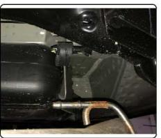
Fishwire (3) CM-SP10 spacers and (3) 1/2" carriage bolts through access hole and out mounting holes on each side of vehicle. (As shown in the Fishwire Technique Diagram) Remove access panel by removing (2) wing nuts. Pull access panel down and away from vehicle. Set aside panel for reinstallation.
