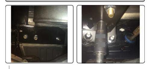
4. Reinstall vehicle bracket hardware and exhaust system as removed in Step 1. When hitch is not in use reinstall access panel removed in Step 2.
