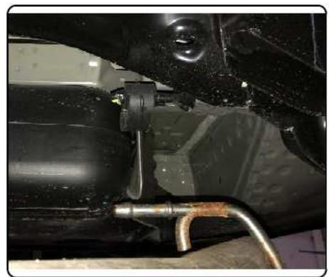
2. Fishwire (3) CM-SP10 spacers and (3) 1/2" carriage bolts through access hole and out mounting holes on each side of vehicle. (As shown in the Fishwire Technique Diagram) Remove access panel by removing (2) wing nuts. Pull access panel down and away from vehicle. Set aside panel for reinstallation.
