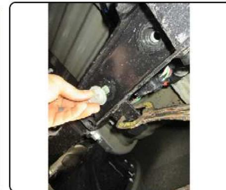
2. Raise hitch and into position, use existing hardware removed in step 1 to secure hitch and assembly to vehicle.
