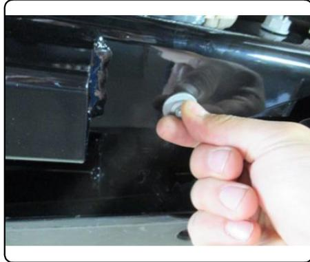
6. Place the Tail Bracket clamp plate (13411-TBC) between the rear differential and the cross member as shown below. Raise the Tail Bracket Weldment (13411-TBWA) into position between the Main Body Weldment and the vehicle cross member. Loosely install the 1/2" fasteners as shown on page 2.
