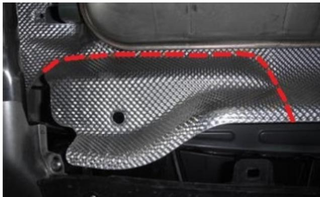
**HEAT SHIELD TRIM DIAGRAM (BOTH SIDES)
