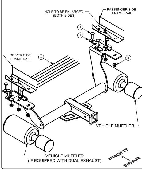
1. Remove (2) exhaust hangers from the passenger side muffler and (1) exhaust hanger from the center front of vehicle for single exhaust vehicles, dual exhaust will remove (2) exhaust hangers from the driver side muffler as well. Support lowered exhaust with jack stand.
