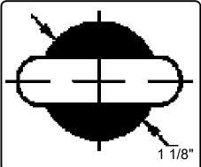
4. Fishwire 1/2" carriage bolt and spacer through the front and rear frame holes in both frame sides then reverse fishwire the center hole both sides. **Optional:** Drill 5/8" clearance holes in heat shield using dimples as guides and reinstall heat shield without rear most frame attachment.
