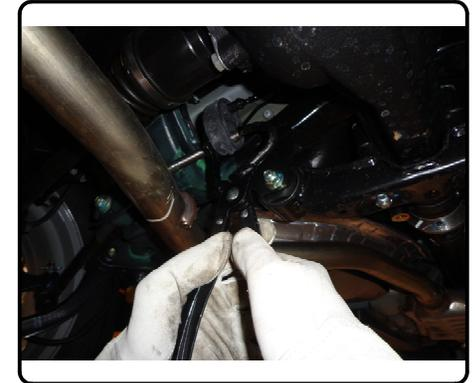
2. Remove (4) heat shield attachments with phillips head screwdriver or 10mm socket (both sides if equipped with dual exhaust and proceed to Step 3). Remove underbody panel from driver side frame rail by removing (2) screws and (5) push fasteners. Save for reinstallation.
