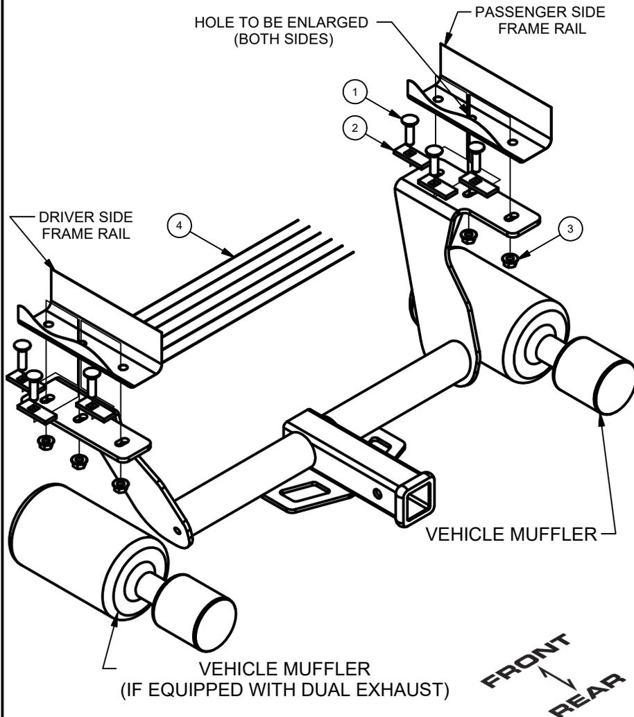
1. Remove (2) exhaust hangers from the passenger side muffler and (1) exhaust hanger from the center front of vehicle for single exhaust vehicles, dual exhaust will remove (2) exhaust hangers from the driver side muffler as well. Support lowered exhaust with jack stand.
