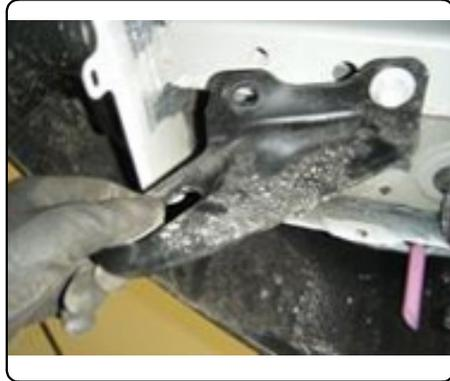
8. Lower exhaust by lowering the rearmost exhaust isolator while supporting the exhaust.
