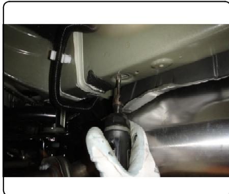
5. Fishwire 1/2" carriage bolt and spacer through the forward-most frame hole into the center and rear frame holes, then reverse fishwire into the forward-most hole for both sides.
