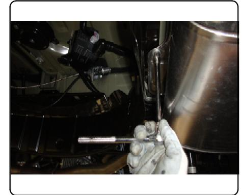
2. Locate and remove the center front attachment point on the spare tire shield using a 12mm socket. Remove the spare tire shield and return to the customer.
