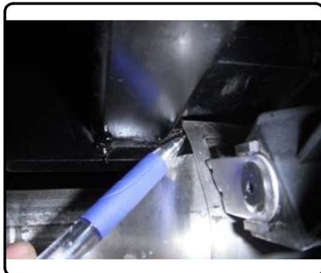
5. Torque 1/2" hardware to 110 lb-ft. Torque M14 hardware to 139 lb-ft (if present).
