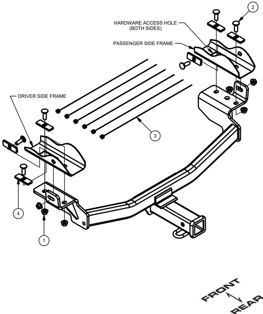
1. Remove the exhaust by removing (2) bolts connecting the exhaust hanger bracket from the frame, using a 13mm socket (Both sides). Using a 15mm socket, loosen the exhaust clamp just forward of the muffler and remove the rear portion of the exhaust from the vehicle. Support exhaust from underneath during install.
