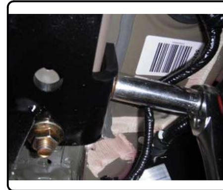
6. Raise exhaust back to original position, and secure exhaust bracket bolts. If present, reattach wire removed in Step (4) to original position.
