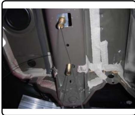
4. Raise hitch into position and loosely secure hitch with the hardware, careful not to push hardware inside vehicle frame. Trimming of exhaust bezel may be required on some models. (Check trim fitment around hitch, additional trimming may be required. Seam foam may need to be trimmed for proper fitment)
