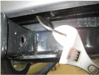
**Note:** Some models may require adjustment to the factory safety chain loops to provide clearance for the hitch pin. Using an adjustable wrench, bend the loops upward as needed. (see photo above)
